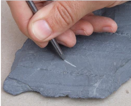
Clay minerals can be scratched by a steel pin (in this photo slate is substituted for marl).
